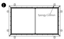
• Before assembling the outer black frame, place the sponge cushion under the assembled screen as per the diagram
