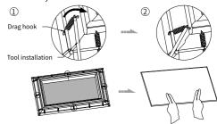
Note: If there is some wrinkles appear, please wear the provided gloves and use fingers to gently press and move on edge area of screen material by left hand to the left side and right hand to the right side.
