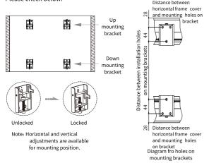
Please make sure the brackets are firmly installed. Hang the screen onto upper mounting bracket and make adjustment until upper bracket is at the middle of screen. Let the screen hanged vertically and tight the screw of down mounting bracket until screw is attached to slot of down frame. Please check below:
