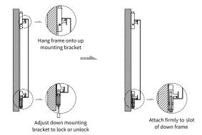
For uninstall of screen, unscrew down mounting brackets till it is loosen from slot of down frame. Lift the screen lightly to make it go off upper mounting bracket and finish uninstall.
