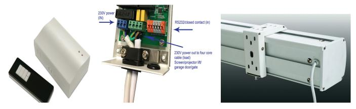
Each Screen over 3M in the Mayfair range comes with a radio frequency control box (40m range) which incorporates an RS232 and zero volt contact closure socket inside. There is a cable from the left hand side of the screen that has approx 1.4M of 4 core cable into the control box. There is then a further 1.4M of three core cable terminating in a UK plug.
